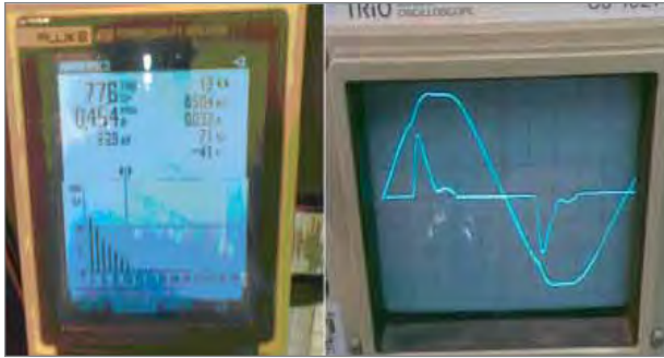
Figures 12 and 13: four CFLs in parallel
