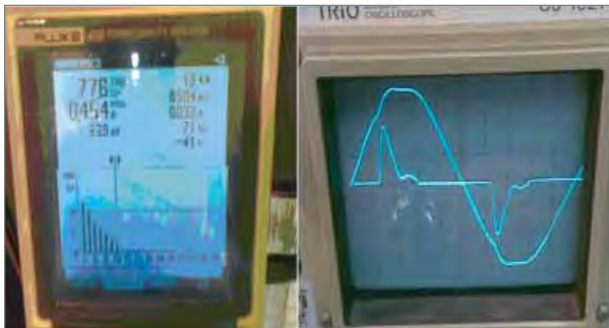
Figures 14 and 15: six CFLs in parallel
