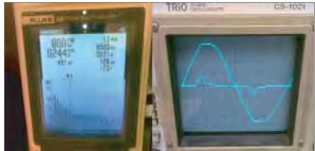
Figures 10 and 11: two CFLs in parallel
